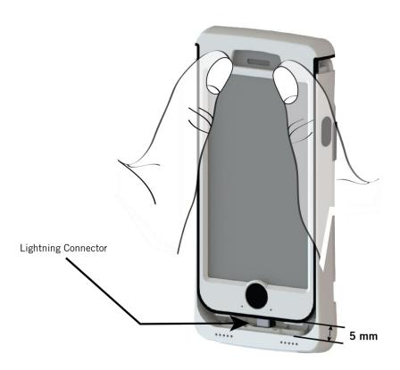
Pull the top plate toward you, away from the bottom carriage. Do NOT try to slide it all the way up.
